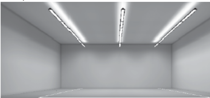
B) Fluorescent T8 in continuous rows
